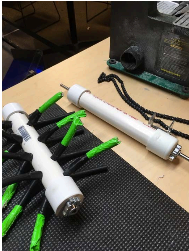
Left: Collector mechanism in progress. Right: Idea for changing the cap ball lift motor setup.
