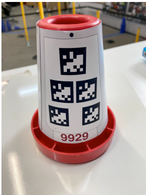
The AprilTags Sleeve proved too sensitive to slight misalignments.
