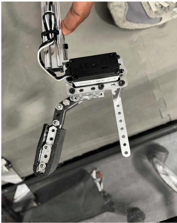
**Final Design:** Through a lot of trial and error we ended up with a gripper for our final design. The gripper was much simpler and proved to be more efficient when picking up samples. It solved our problem of not being able to pick up samples unless directly touching the sample. The gripper does not have to be perfectly lined up with the sample to be able to pick it up, it can be at an angle or even pick the sample up horizontally.
